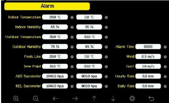
Figure 36: Alarm Setting Screen
