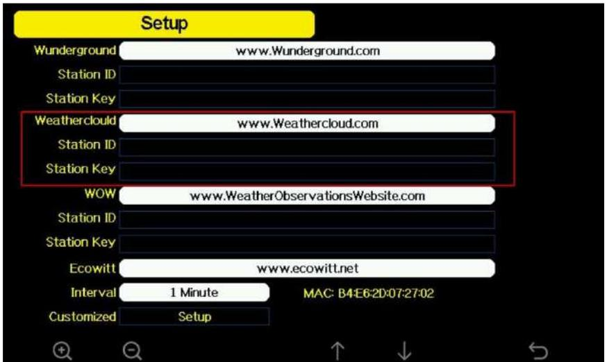
Figure 31: Weathercloud Server setup screen
